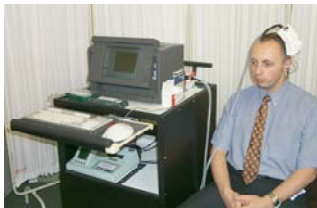
The non-invasive ICP assessment being performed on a volunteer. The system is PC based and uses a headset to deliver the sound and measure the tympanic membrane displacement with a simple tympanometer probe placed in the ear canal.
